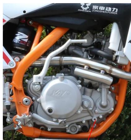
and wheels should be cleaned. Check the replaced coolant, if there are white spots in the coolant, it means that the aluminum-containing part of the cooling system has been corroded. If
