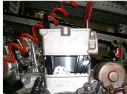
Clean the remaining gaskets on the cylinder surface with a spatula
