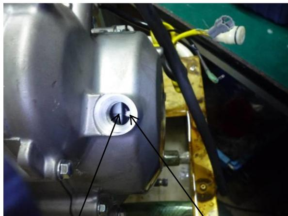
NC250 Magneto rotor timing mark
