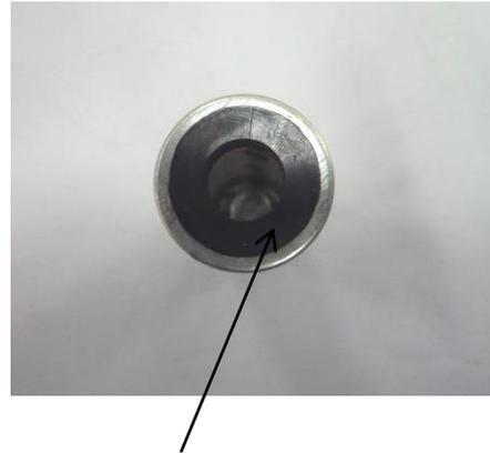
Open end of oil filter, facing left box when assembling
