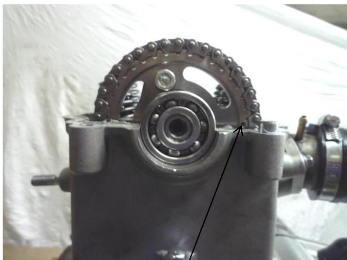
Timing driven sprocket timing mark
