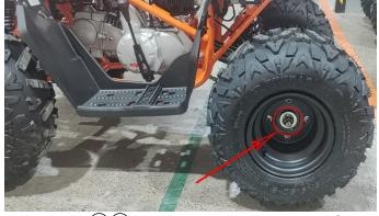
8.Use tool (1)(3) to remove the rear wheel fixing screws.
