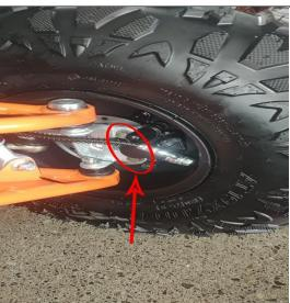
3.Use tool (9) to remove the disc brake pump fixing bolts.
