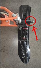
7.Install A to the front wheel hub mounting shaft, put D through the front disc brake mounting hole with E to the front disc brake pump. Then install the nut removed before from the front wheel back on the front wheel shaft.
