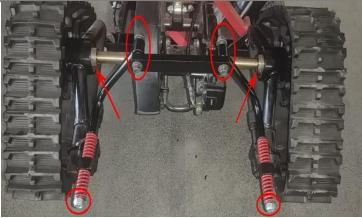
11.Put F G to the rear axle, assemble H J L together and put it to the mounting hole of the roll rod on the track assembly, then put an anti-roll spring and a gasket and use P to settle them. The other end connected with M and O.
