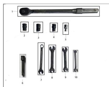
1. The above picture shows the tools required for assembling the kit.
