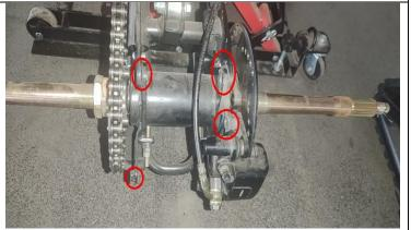
9.Use tools 78 to remove the fixing bolts from the rear axle barrel, then use tools 90 to remove the fixing bolts from the disc brake pump and the chain cover.
