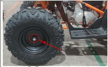
4.Use tool ① ③ to remove the front wheel fixing bolts.
