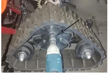
12.Install the nut removed before from the rear axle back into the rear track and lock it with tools (1)(3).
