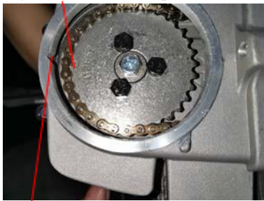
Timing mark of cylinder head Magneto rotor timing scale
