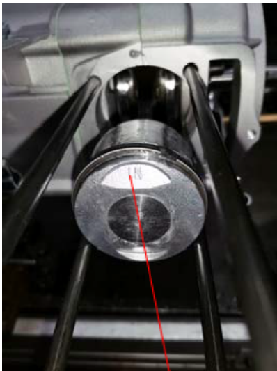
“IN” side of intaking air
