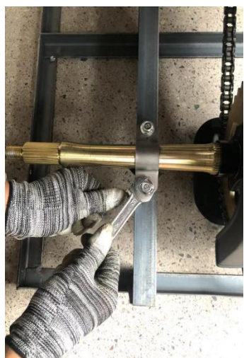
10. Use tool ⑨⑩ to remove the fixing screws of the iron frame.
