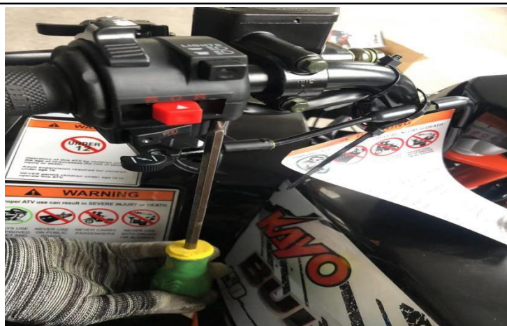
9. Use tool ⑫ to install the combination switch
