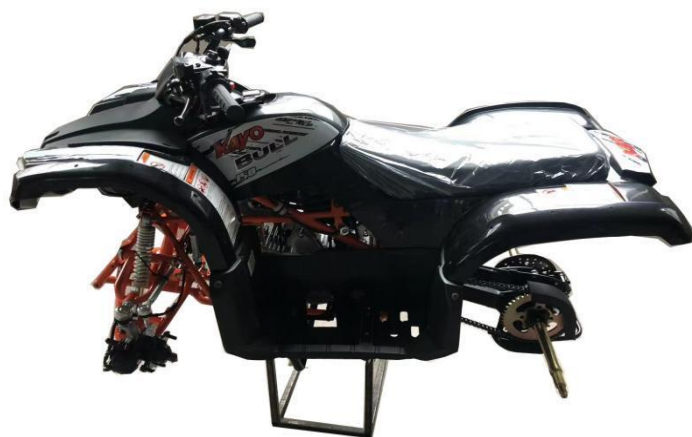
11. Put the vehicle on the stand for easy installation of other accessories.
