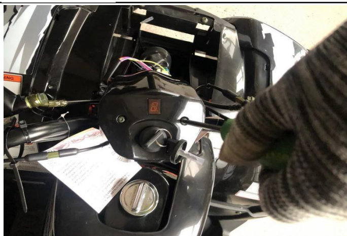
8. Use tool ⑫ to tighten the gear indicator screw (S).
