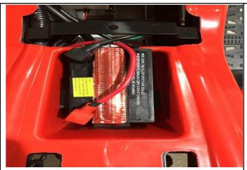
21.Connect the positive and negative poles as shown above, use tool (10) to tighten the bolts and re-install the seat.
