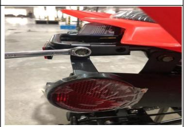
14.Use tool (8) to install the reflector(G) with bracket and screws in the position shown above.
