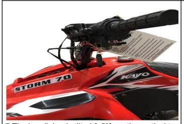
7. The handlebar is tilted 3-5° from the vertical to the rear after installation.
