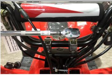
6. Use tool ① ⑤ to lock the Handlebar upper clamps(K), the distance between the two ends of the mark is close, tighten evenly, first start by hand tightening all four clamp bolts
