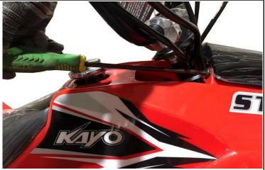
22.Use tool 10 to install the head cover(C) and bolts & washers(L).
