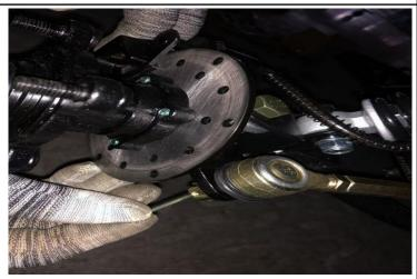
12.Use tool ①⑥ to tighten the nut of the steering pull rod(M) and insert the cotter pin. Please make sure the bending angle is greater than 180°. Note: Torque requirement 49-59N.m
