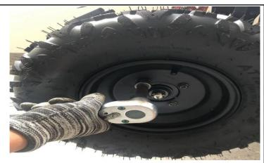
16.Install the front wheel on the front hub, use tool ①③③ to tighten the nut(E).
