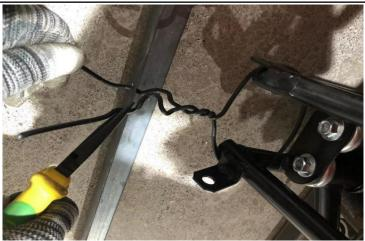
8. Remove the iron wire fixing the front frame and the packing frame.
