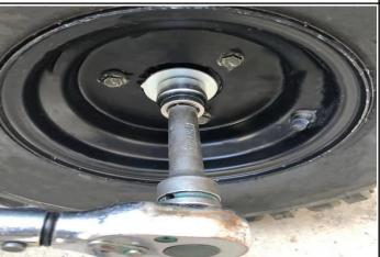
17.Align the rear wheel with the splines and push on the rear axle, with the air nozzle cap facing outward. Use tool ①②③ to lock the nut and washer, then insert the cotter pin(D), keep the bending angle greater than 180° Note: Torque requirement 77-92N.m
