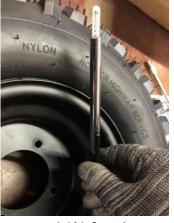
15.Please refer to user's manual (A) for air pressure requirements. Use compressed air to inflate the tires, and use the air pressure gauge (H) to inflate to the standard value of 5psi.
