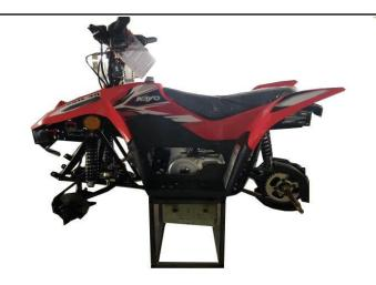
10.Put the vehicle on the stand for easy installation of other accessories.
