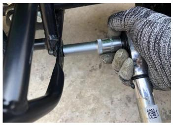
13.Use tool ①④ to tighten the bumper fixing bolts(F).
