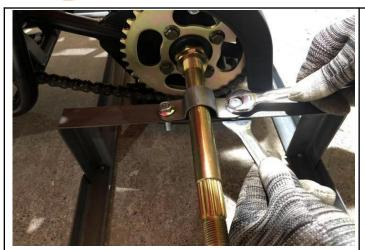
9.Use tool 89 to remove the bolts that fix the rear wheel axle and the packing frame.
