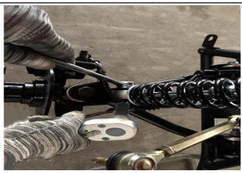
11.Use tool ①③⑦ to tighten the front shock absorber bolts(N).
