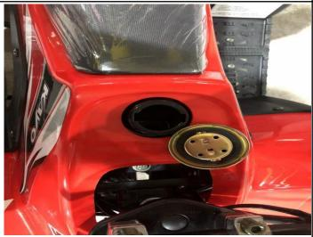
23.Unscrew the fuel tank cap, add gasoline, then tighten the fuel tank cap clockwise.
