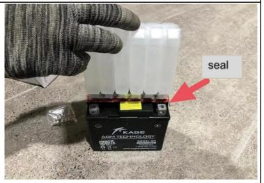
20. Take out the battery, according to the user's manual (A), first tear off the seal on the battery, add electrolyte, then install the battery cover and wait for the subsequent installation into the battery box.
