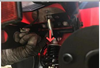
19.Pull the latch as above shown and remove the seat cushion, waiting for the subsequent installation of the battery.
