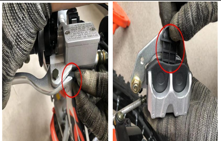
13. Use tool ⑭ to remove the fixing bolt of the caliper of the front brake, and remove the plastic buckle.
