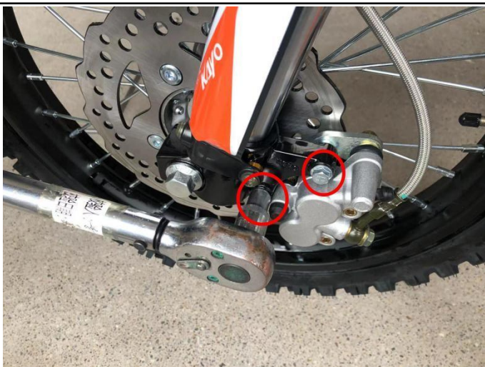
14. Use tool ①⑤ to tighten the fixing bolts of front brake caliper (torque: 10-12 N.m).
