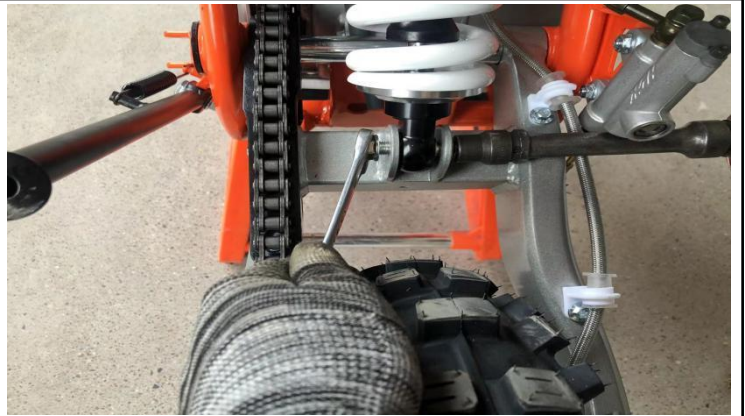
11. Use tool ①②⑦⑫ to tighten hexagon flange bolts M10*45 and hexagon flange lock nut (torque: 49-59N.m).
