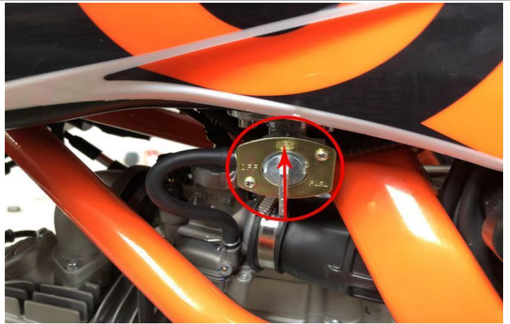
23. Turn the fuel tank petcock to the position shown as above.
