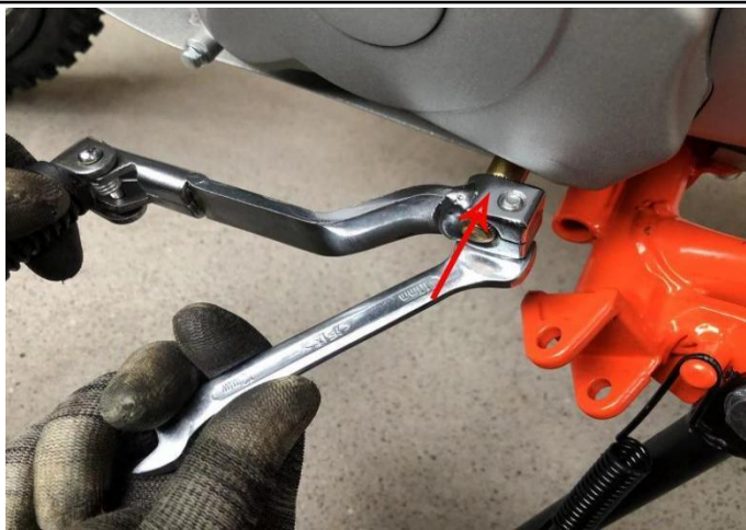
16. Insert the gearshift lever (F) into the gear shaft, then use tool ⑪ to tighten the screw.
