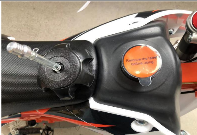
24. Install the fuel tank cap (I) with vent valve (O) together, then fill in fuel and tighten the tank cap.
