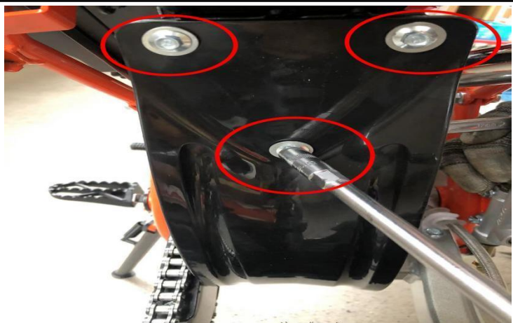
21. Install rear shock mud fender (B) on the battery box, use tool ⑰ to tighten the bolt M6*16, washer \Phi 6 \times 18 \times 1.5 and nuts M6 (N).
