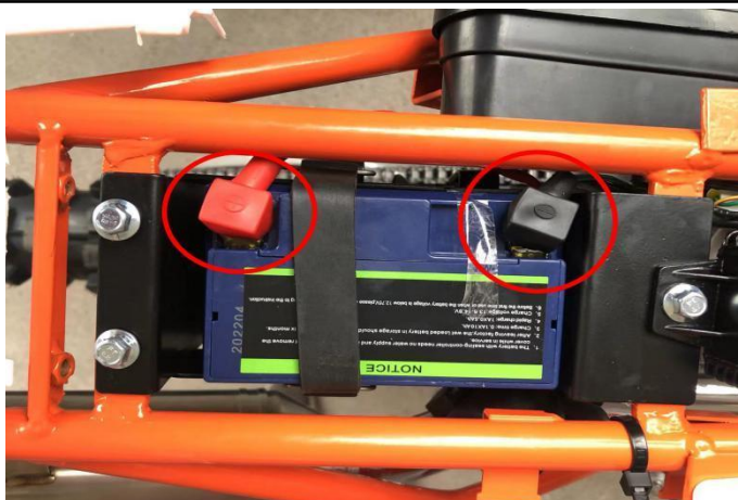
Put the battery into battery box, and fix it with belt (G), then use tool ⑮ to tighten the battery screw (red is positive, black is negative). Finally, install the seat.
