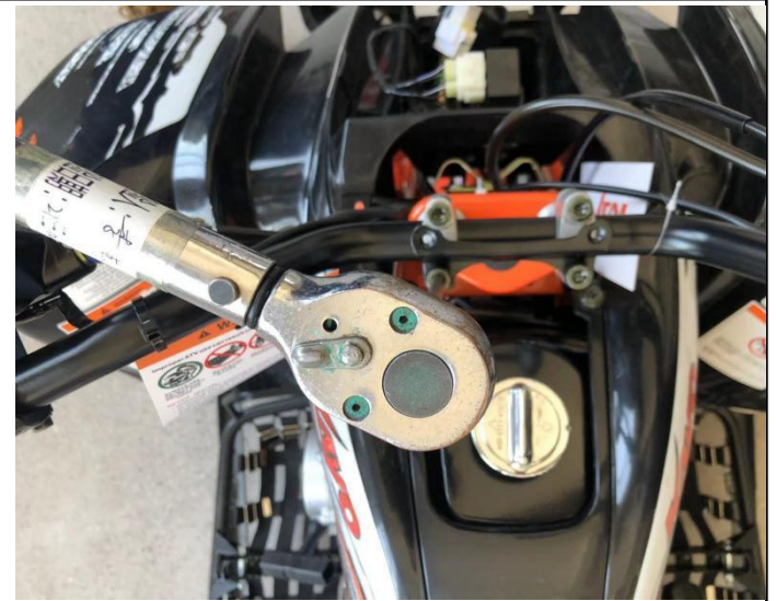
7. Install bracket for gear indicator cover(F), use tool ①③ to tighten handlebar clamps, the distance between the two ends of the mark is close, tighten evenly, first start by hand tightening all four clamp bolts. (The handlebar is tilted 3-5° vertically to the rear after installation, and the torque is required to be 25-30N.m)
