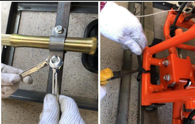
10. Use tool ⑩⑫ to remove the screws fixed on the rear axle, and then use tool ⑧ to remove the screws fixed to the front of the frame (The front frame fixing wire is a temporary solution, and the subsequent packaging is fixed with bolts)
