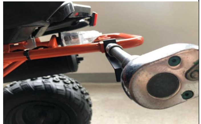
25. Take out rear L&R reflector bracket(C) from the accessory box and use tool ①⑤⑨ to tighten the screws(T) of the reflector bracket and install the reflector. (torque requirement 25-30N.m)
