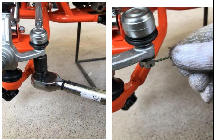
13. Install the pull rod on the steering knuckle, then install slotted nut and washer(K). Use tool ①④ to tighten, and insert the cotter pin(K), the bending angle is greater than 180°(torque requirement 49-59N.m)
