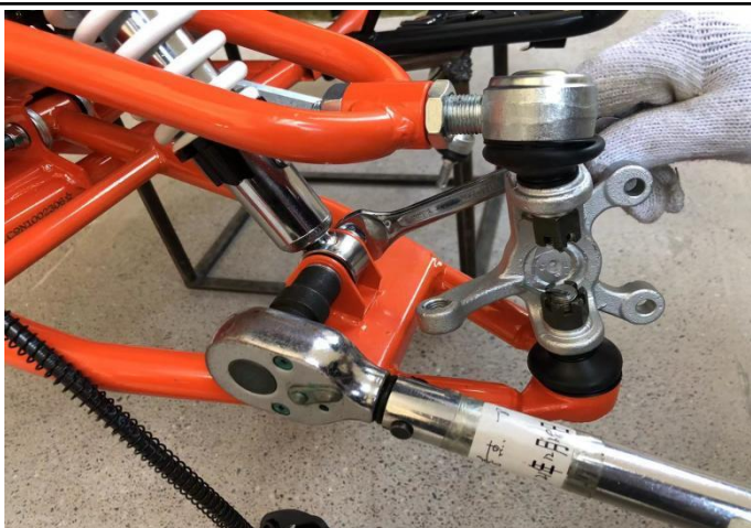
12. Use tool ①⑫⑯ to tighten front fork bolt and nut(L). (torque requirement 49-59N.m)
