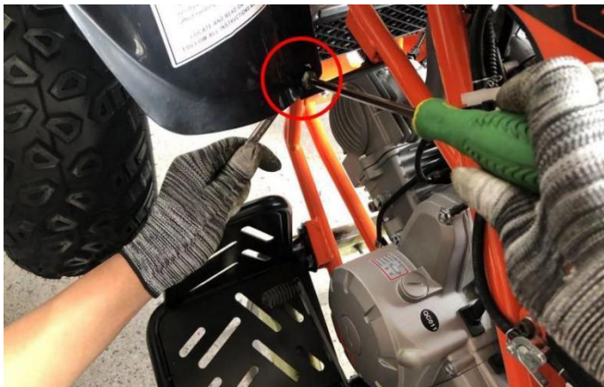
24. Use tools ⑦⑩ to tighten the front plastics screw, washer and nut(Q)
