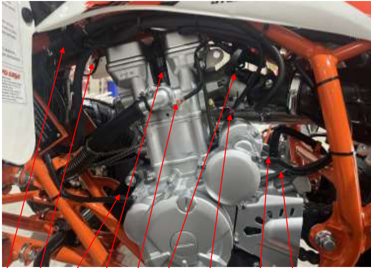
1. Oil pipeline 2. Fuel pump 3. Fuel pump connector
