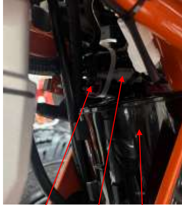
1. High-voltage transformer 2. Carbon Canister 3. Carbon Canister solenoid valve 4. Carbon Canister solenoid valve connector
