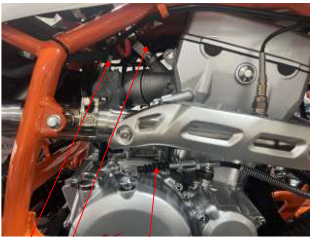
4. Accelerator Cable; 5. Fuel Injector; 6. Clutch Cable
