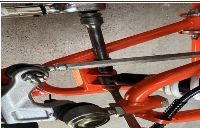
11. Use tool ①②⑥⑬ to tighten the bolts and nuts for the front shock absorber(G)(torque requirement is 49-59N.m).
