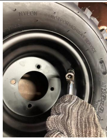
14. Please refer to user's manual (A) for air pressure requirements. Use compressed air to inflate the tires and use the air pressure gauge (E) to inflate to the standard value of 5psi.
