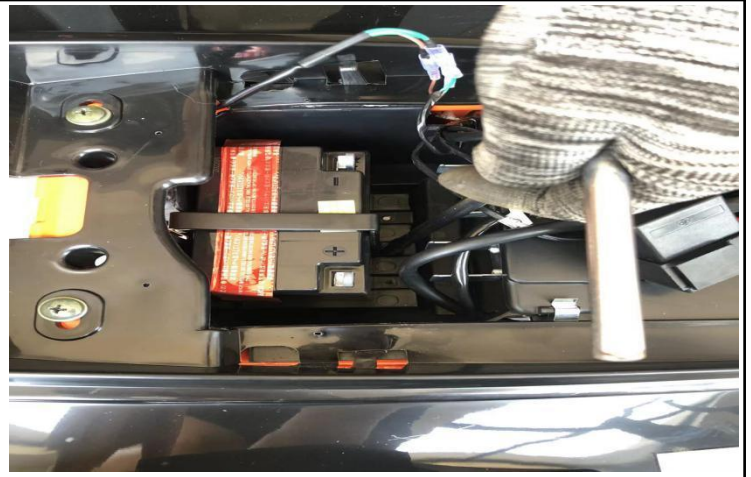
20. Use tool ⑩⑭ to remove the battery fixing bracket, put in the battery and install the fixing bracket back.
