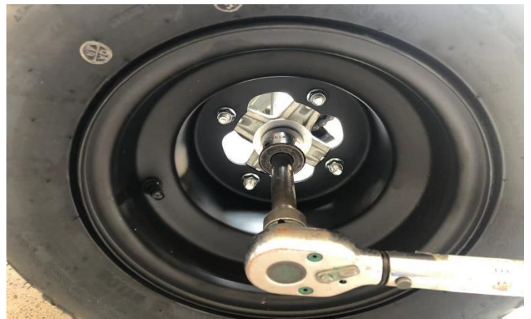
16. Align the rear wheel with the splines and push on the rear axle, with the air nozzle cap facing outward. Put on the nut/washer/spring washer first then insert the cotter pin(K), keep the bending angle greater than 180° (torque requirement 86-103N.m).
