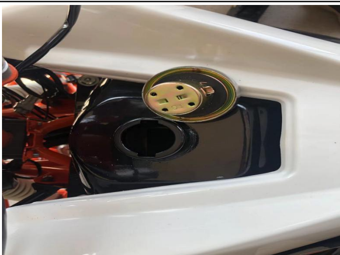
23. Unscrew the fuel cap, add gasoline, and tighten the fuel cap clockwise.
