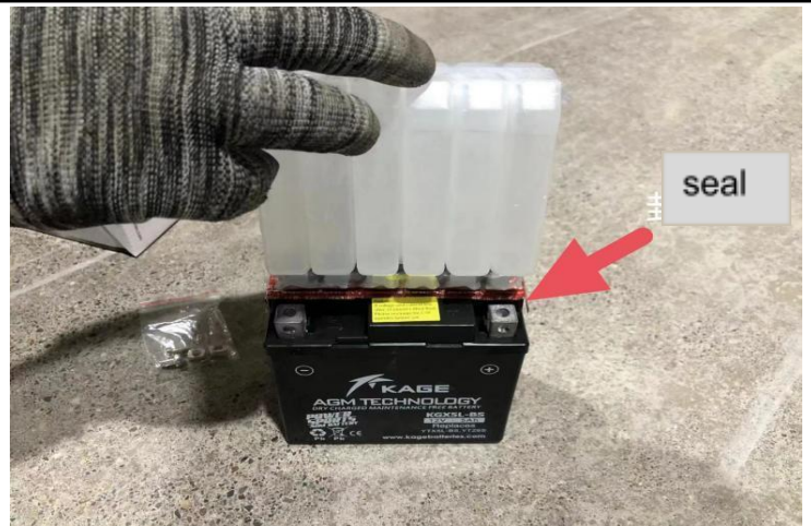
18. Take out the battery, according to the user's manual (A), first tear off the seal on the battery, add electrolyte, then install the battery cover and wait for the subsequent installation into the battery box.
