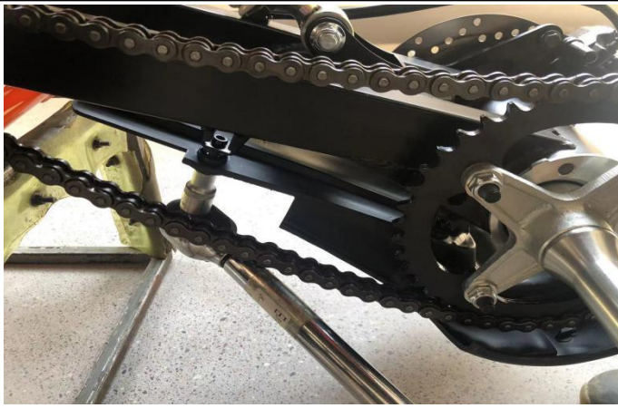
13. Use tool ①④⑫ to tighten the bolts for the swing arm protector(J).
