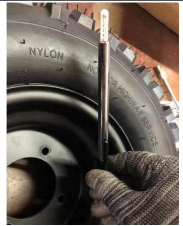
14. Please refer to user's manual (A) for air pressure requirements. Use compressed air to inflate the tires and use the air pressure gauge (E) to inflate to the standard value of 5psi.
