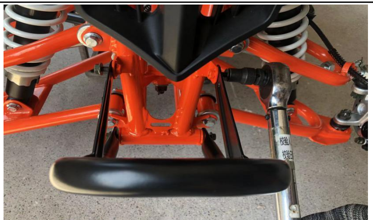
12. Use tool ①⑤ to tighten the bolts for the Front bumper(H)(torque requirement is 25-30N.m).
