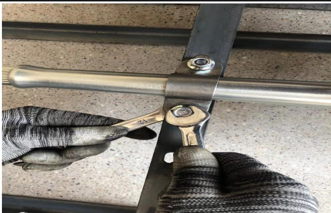
9. Use tool ⑪⑫ to remove the bolts that fix the rear wheel axle and the packing frame.
