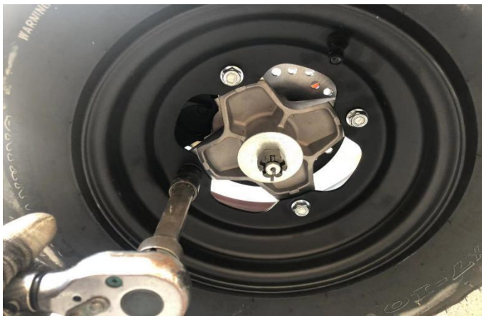
15. Install the front wheel on the front hub, use tools ①②⑥ to tighten the bolts(F) (torque requirements 49-59N.m).
