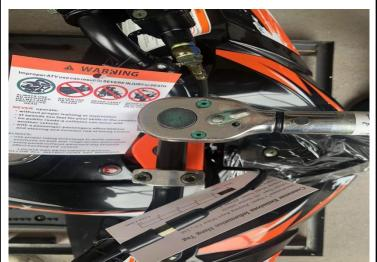
6.Use tool ① ⑤ to lock the handlebar upper clamps, the distance between the two ends of the mark is close, tighten evenly, first start by hand tightening all four clamp bolts.
