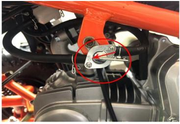
20. Rotate the petcock to the direction of the arrow as shown above.
