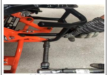
13.Use tool ①④⑧⑫ to tighten bolts and nuts(L) for the front guard.
