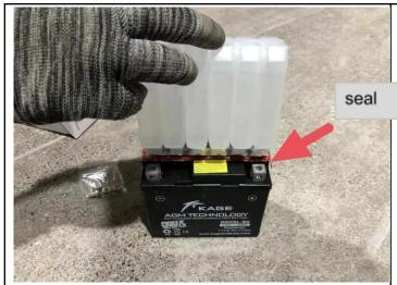
17. Take out the battery, according to the user's manual (A), first tear off the seal on the battery, add electrolyte, then install the battery cover and wait for the subsequent installation into the battery box.
