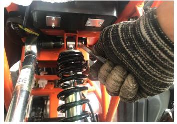
7. Use tool ①②⑦ to tighten the rear shock absorber bolt & nut(O).
