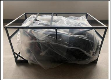
3. Take out the parts attached on the vehicle and the packaging iron frame, remove the iron frame screws, wait for subsequent installation.
