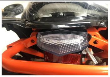
9. Use tool ① to tighten the nuts and washers (M) for rear reflector(D) and taillight.
