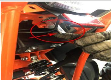
18.Pull the latch as above shown and remove the seat cushion, waiting for the subsequent installation of the battery.
