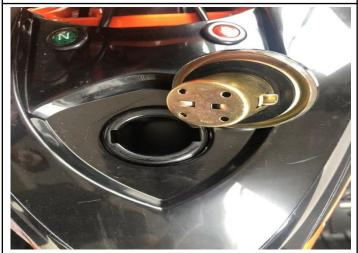
21.Unscrew the fuel cap, add gasoline, and tighten the fuel cap clockwise.
