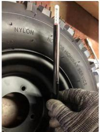
14.Please refer to user's manual (A) for air pressure requirements. Use compressed air to inflate the tires, and use the air pressure gauge (B) to inflate to the standard value of 5psi.
