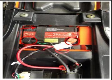
19.Install the battery and fix it with H. Connect the positive and negative poles as shown above, use tool ① to tighten the bolts and re-install the seat.
