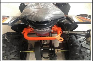
10.Use tool ①④⑫ to install the bracket(J) and tighten the bolts(P) first, then install the right/left reflectors.
