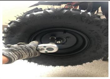
15.Install the front wheel on the front hub, use tool ①② to tighten the nut(N).
