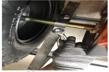
8. Use tool (8) to remove the fixing bolts of the iron frame and the rear axle.
