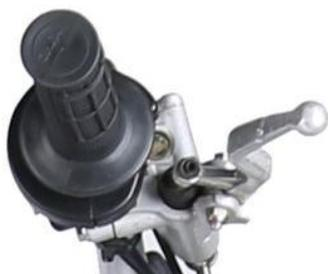
The front disc brake is controlled by the brake lever. Which located at the right end of the handlebar, and operated by the right hand.
