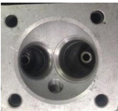
Completely remove the carbon deposits in the combustion chamber, apply a thin layer of red stamping oil evenly on the valve seat, place the valve on the valve seat and knock the valve lightly without rotating, and then pull out the valve. If the contact marks on the valve working surface are discontinuous, the valve seat should be polished and repaired.
