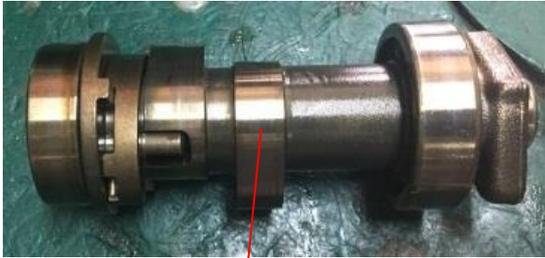
The camshaft convex hull has no obvious unevenness when touched by hand
