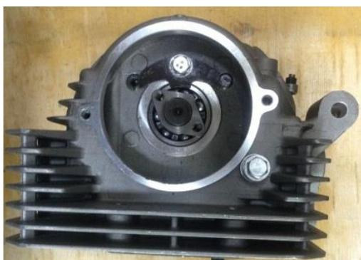
1. Remove the camshaft limit bolt;
