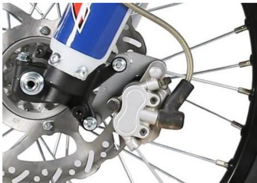
The front brake adopts a floating caliper disc brake, which is installed on the lower end of the left front shock and fixed by 2 bolts.
