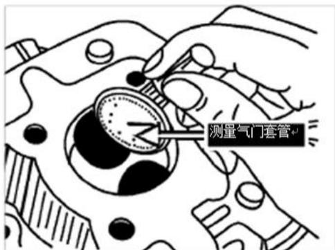
Use a dial indicator to measure the inner diameter of each valve catheter and make a record. Repair limit value:  $\phi 5.035$  mm
