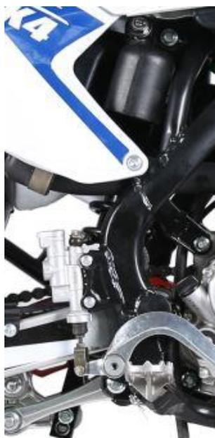
Check the rear shock absorber whether the airbag is normal and the spring is cracked or not, etc. If necessary, replace the rear shock absorber.
