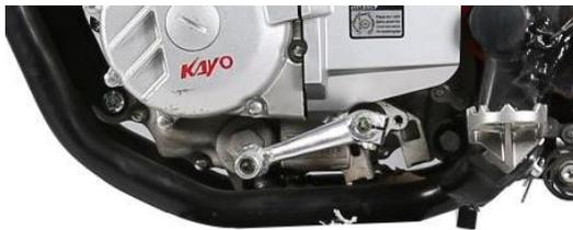
The K4 shift lever is located on the left side of the engine, and the shift operation is performed by stepping on and hooking up the shift lever.
