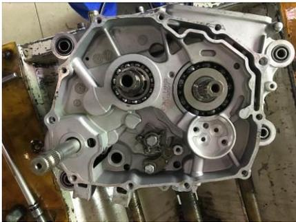
1. First install the O-ring of the oil pump on the box;
