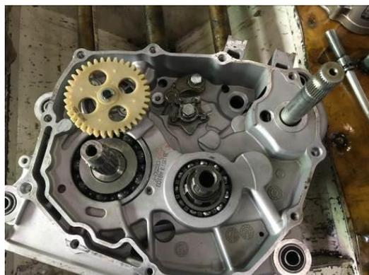
1. Remove the oil pump fastening screws;
