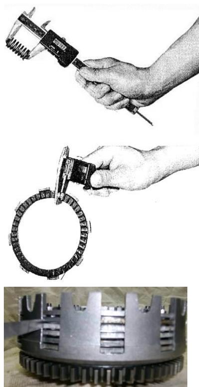
1. Measure the free length of the clutch spring
