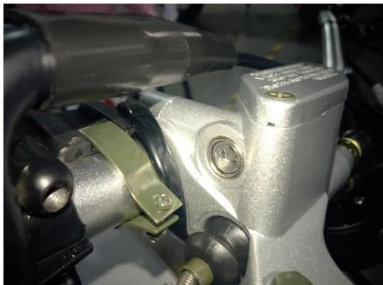
K4 model use hydraulic disc brakes, and the brake fluid level of the disc brakes can be checked through the observation hole.
