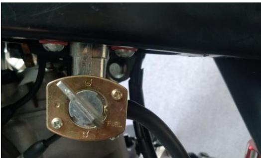
The K4 carburetor version adjusts the fuel supply through the fuel tank switch, which is located at the bottom of the left side of the fuel tank. By rotating the switch, you can control whether the fuel enters the carburetor, so as to achieve the control effect.
