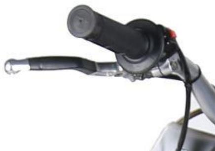
The clutch is controlled by the clutch lever, which is located at the left end of the handlebar, and operated by the left hand.
