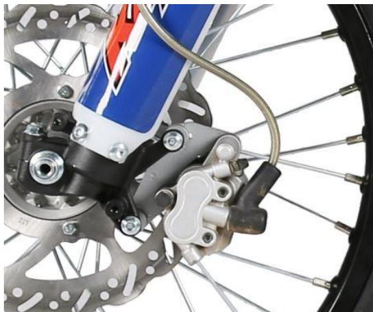
The disassembly and installation steps of the front disc brake are as follows:
