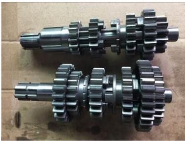
Check whether the gears of the main and countershaft assemblies have excessive or abnormal wear, and check whether the collars between the gears are deformed or fallen off.
