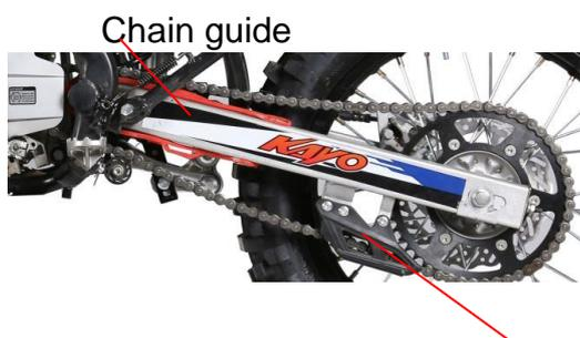
Check the wear of the chain guide and the chain protector on the swingarm. Under normal circumstances, these two can play a role in guiding the movement of the chain. If the wear is too large, it is not conducive to the normal movement of the chain and affects its transmission effect. Therefore, the excessively worn chain guide and
