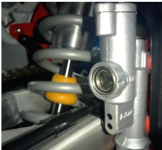
Observe through the liquid level hole to check the level of brake fluid. The liquid level should exceed half of the observation hole, that is, the liquid level should be higher than "LOWER". If the brake fluid is insufficient, it should be added immediately.
