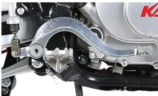
The foot brake pedal is located on the right side of the engine and is operated by stepping on it.
