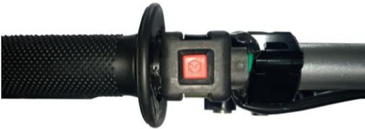
The engine's flameout switch is located on the left side of the handlebar near the grip. It is a square red button. Long press it to turn off the engine.
