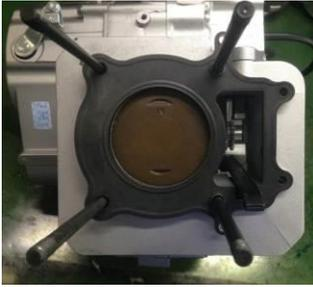
1. Remove the cylinder head gasket combination;
