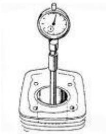
1. Check whether the cylinder block is worn or damaged;
