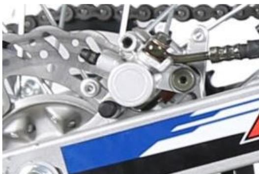
The rear wheel brake adopts a floating caliper disc brake, whose caliper body is located on the right side of the rear wheel and is fixed by a disc brake bracket.
