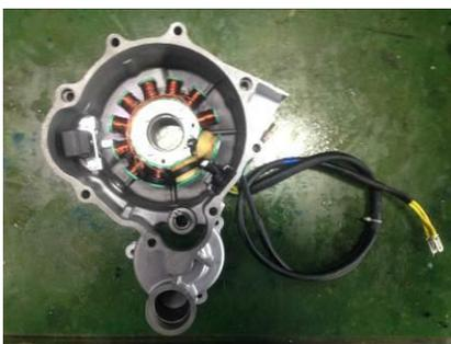
1. Install the magneto stator assembly to the left crankcase cover.
