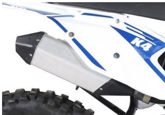
The exhaust pipe and the muffler can guide the gas emission and reduce the noise.
