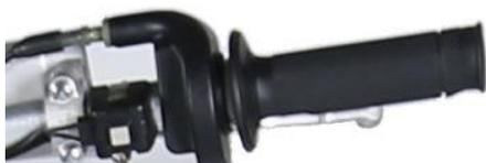
The throttle knob is located on the right side of the handlebar and is controlled by turning with the right hand. When the handle is turned counterclockwise, increase the throttle, release the handle and return it to the position.
