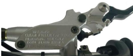
The brake fluid must be checked and replaced regularly. If the brake fluid is mixed with water, soil or other particles, the brake fluid should also be replaced.
