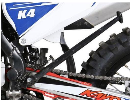
K4 use a single support for parking support. The single support is located on the left side of the whole vehicle. When in use, the vehicle is centered and the single support is kicked to expand it. Tilt the whole vehicle to the left to make the single support contact the ground and support the motorcycle.
