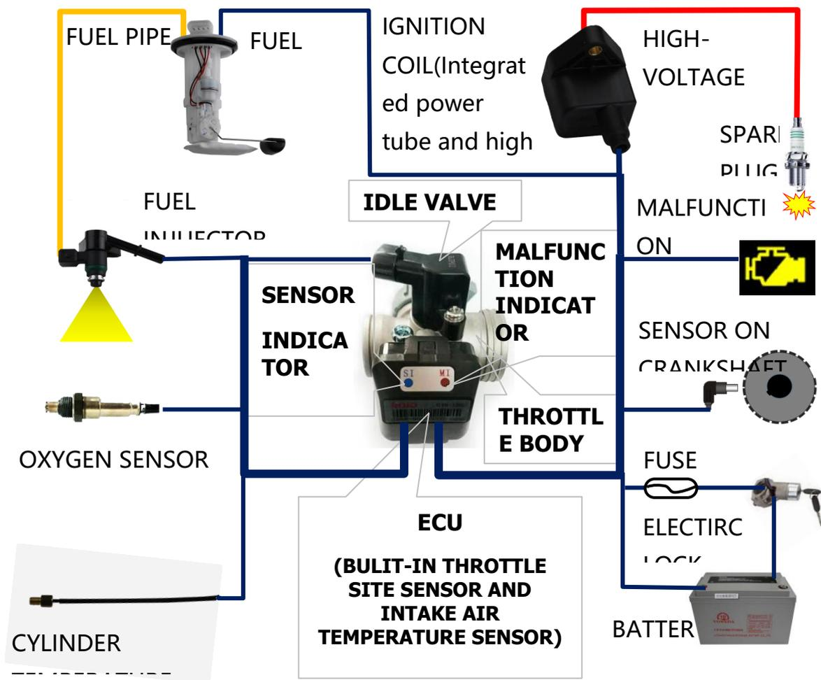
PIC.1: SCHEMATIC DIAGRAM OF EFI SYSTEM
