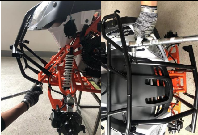
12. Use tool ⑩⑪ to install front rack and front fence tighten O & S (the torque is required to be 25-30N·m)
