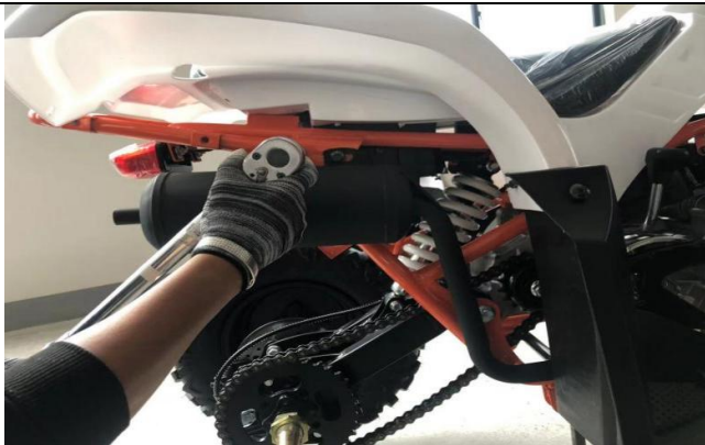
14. Install subframe as above, use tool ⑩⑪ to tighten Q (torque is required to be 25-30N·m).
