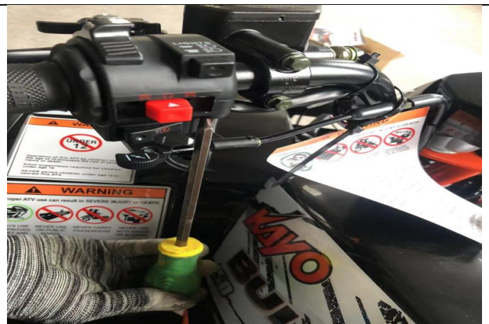
9. Use tool ① to install the multi-functional switch.
