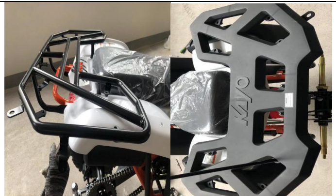
15. Install rear rack as above use tool ⑩⑪ to tighten P (torque is required to be 25-30N·m). Then use ⑩ to tighten P for the rear rack cover.
