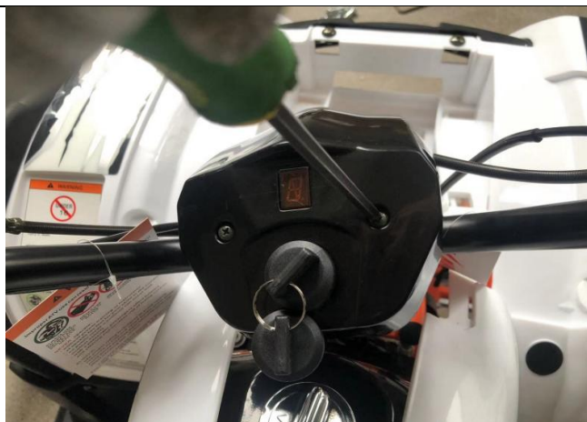
8. Use tool ① to tighten the gear indicator cover bolts.
