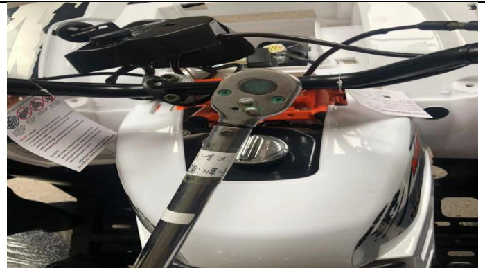
7. Install E, use tool ⑥ to tighten clamps, the distance between the two ends of the mark is close, tighten evenly, first start by hand tightening all four clamp bolts. (The handlebar is tilted 3-5° vertically to the rear after installation, and the torque is required to be 25-30N·m).
