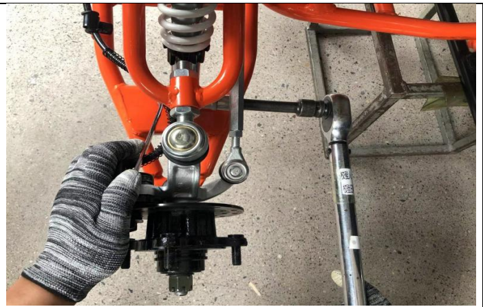
11. Use tool ⑤⑨⑩ to tighten L as above. (the torque is required to be 49-59N·m)
