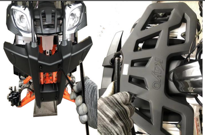
13. Use tool ⑩ to tighten O & S for front rack cover and front fence cover.
