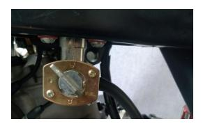
The K2 carburetor version adjusts the fuel supply through the fuel tank switch, which is located at the bottom of the left side of the fuel tank. By rotating the switch, you can control whether the fuel enters the carburetor, so as to achieve the control effect.
