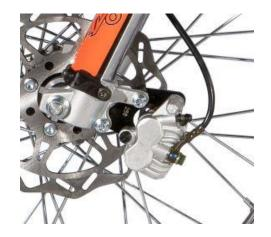
The front brake adopts a floating caliper disc brake, which is installed on the lower end of the left front shock and fixed by 2 bolts.
