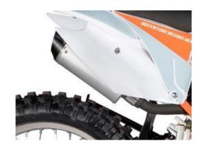
The exhaust pipe and the muffler can guide the gas emission and reduce the noise.
