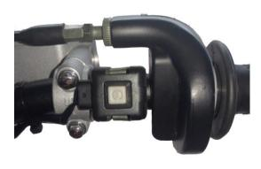
The vehicle start button is located on the right side of the handlebar, close to the position of the throttle knob. It is a square gray button. Long press it to start the motorcycle engine. In addition to the start button, the vehicle can also be started by stepping on the start lever.
