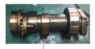
The camshaft convex hull has no obvious unevenness when touched by hand
