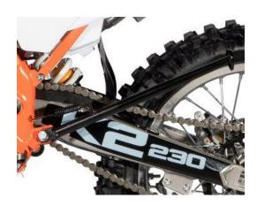
K2 use a single support for parking support. The single support is located on the left side of the whole vehicle. When in use, the vehicle is centered and the single support is kicked to expand it. Tilt the whole vehicle to the left to make the single support contact the ground and support the motorcycle.
