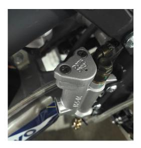
The steps for replenishing rear brake fluid are as follows:
