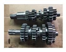
Check whether the gears of the main and countershaft assemblies have excessive or abnormal wear, and check whether the collars between the gears are deformed or fallen off.
