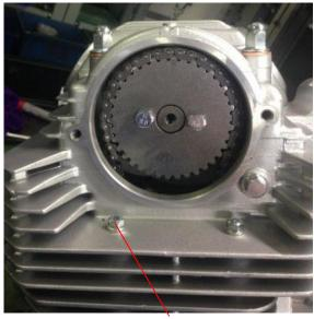
Cylinder head and cylinder block connecting bolt
