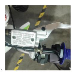
The brake fluid must be checked and replaced regularly. If the brake fluid is mixed with water, soil or other particles, the brake fluid should also be replaced.
