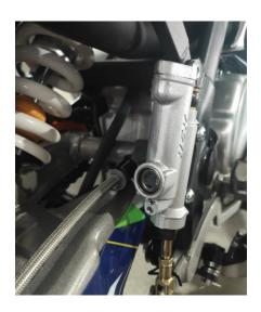
Observe through the liquid level hole to check the level of brake fluid. The liquid level should exceed half of the observation hole, that is, the liquid level should be higher than "LOWER". If the brake fluid is insufficient, it should be added immediately.
