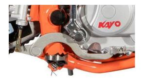
The foot brake pedal is located on the right side of the engine and is operated by stepping on it.
