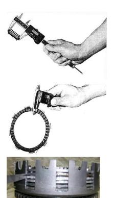
1. Measure the free length of the clutch spring
