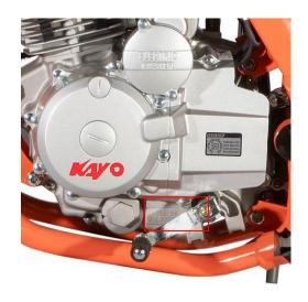
The engine number of the K2 is located on the inside of the engine gearshift lever.
