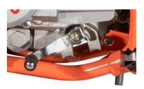
The K2 shift lever is located on the left side of the engine, and the shift operation is performed by stepping on and hooking up the shift lever.
