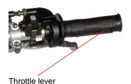
The method of checking the throttle cable is as follows:
