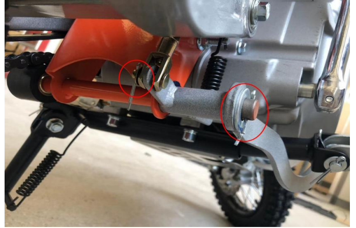
17. Install the end of the pedal to the rear brake as above, then install the washer and cotter pin (the cotter pin is bent at an angle greater than 180^\circ )
