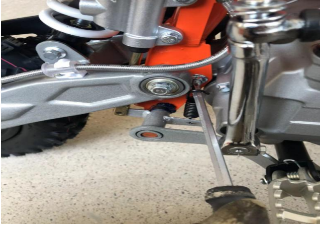
16. Install Q to the frame, use tool ⑥ to install P to the frame.
