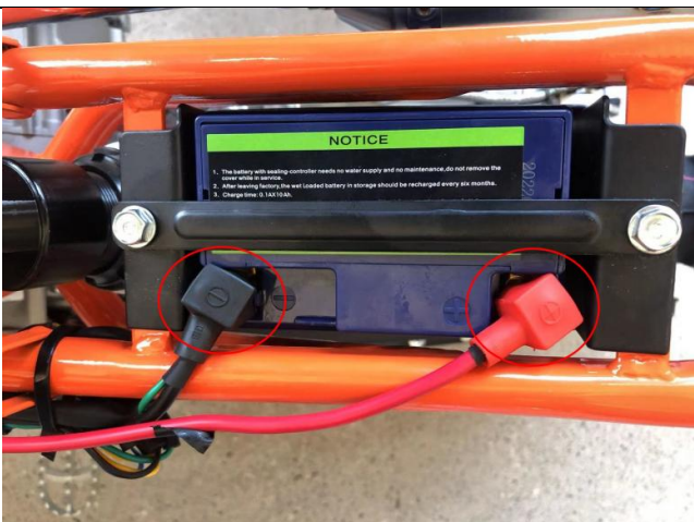
20. Put H&B on the frame together, use tool ⑫ to fix M&N, then use tool ⑥ to install the battery screws. After the installation is complete, install the previously removed seat cushion and plastic fixing screws back (red is positive, black is negative).
