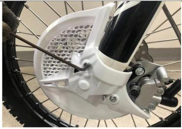
14.Install the front disc brake cover to the left shock and tighten the screws with tool (3)
