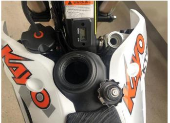
17.Use ratio mix jar to mix the 2-stroke oil and fuel at a ratio of 30:1, add it to the fuel tank and tighten the fuel tank cap. Fill the radiator up with coolant and tighten radiator cap.
