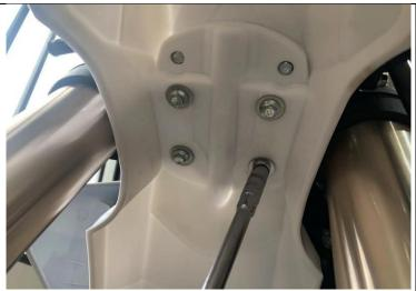
10.Use tool 8 to remove screws of lower clamp assy, then install the front fender and tighten the screws.
