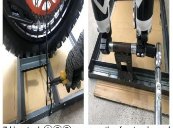
7.Use tool (1)(5)(7) remove the front axle and cut the wire holding the rear wheel.
