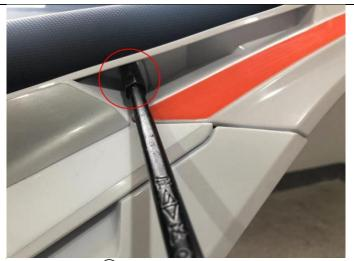
15.Use tool 9 to remove the screws on seat then remove the seat.
