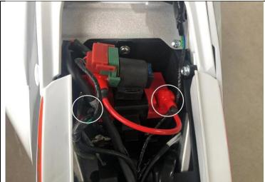
16.Put the battery in and use tool ②to install the battery screws (red is positive, black is negative). Use tool ③ to install the seat.
