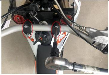
6. Remove the cable tie from handlebar. Use tool ① ⑥ to tighten the handlebar clamps, tighten evenly, first start by hand tightening all four clamp bolts then (torque: 25-30N.m). Install the lower screw of headlight last.
