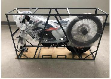
3.Take out the parts attached to the vehicle and iron frame, remove the iron frame screws, wait for subsequent installation.
