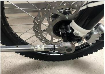
12.Install the front axle then use tool ①5 to tighten the fixing nut. (bushings are on the left, torque: 80-90N.m).
