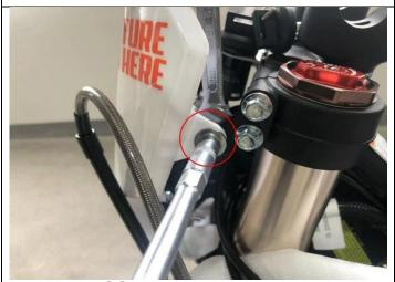
5.Use tool 48 to remove the screw on the left side of headlight, then pull the brake oil pipe out.
