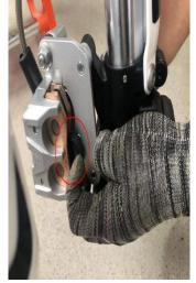
11.Remove the plastic wedges between the front brake lever and between the brake pads .
