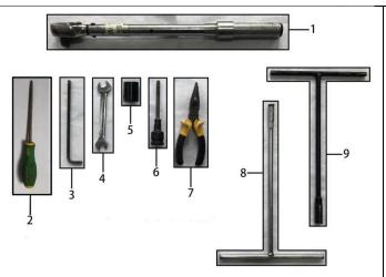
1.Tools for opening and assembling the dirt bike.
