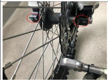
13.Use tool 16 to tighten the screws of front shock at the torque of 25-30 N.m.
