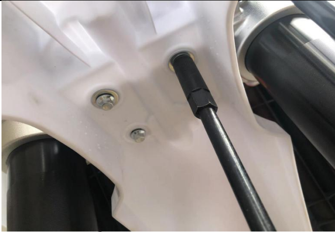
10. Use tool ⑩ to remove the front fender fixing screws, install B and tighten the screws back.
