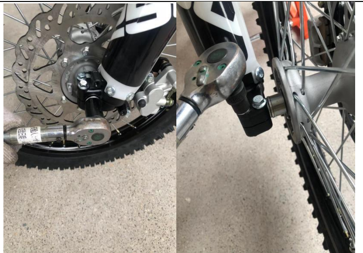
15. First use tool ⑩④ to install D (torque requirement 80-90N.m) (the bushing is long on the left and short on the right), then use tool ⑩③ to lock the front shock absorber screw (torque requirement 25-30N.m)
