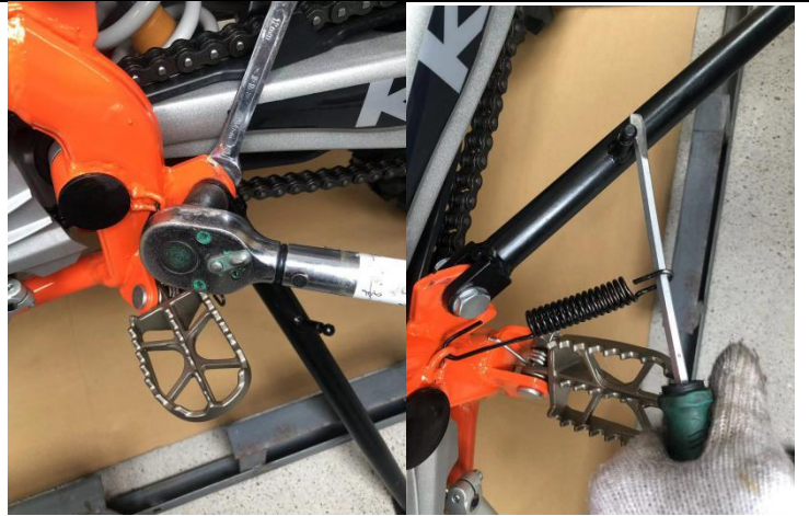
11. Use tool ⑤⑦⑨ to install C (Torque requirement is 20-30N.m).
