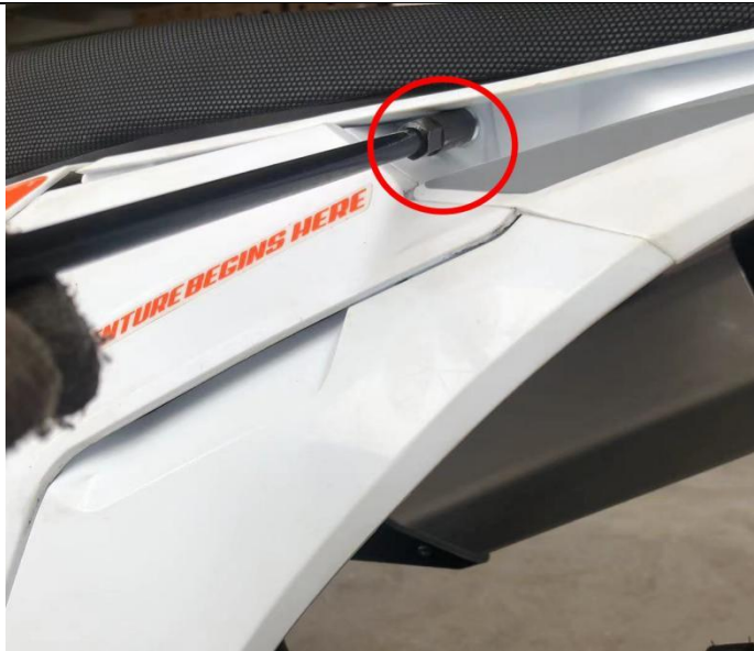
18. Use tool ⑩ to remove the fixing screws on the left and right sides of the seat cushion and remove it for subsequent installation of the battery.
