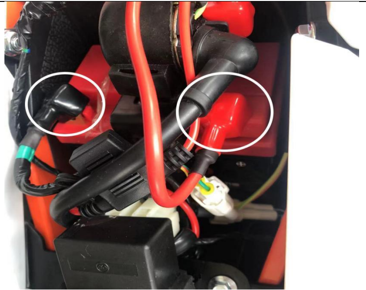
19. Use tool ⑨⑩ to install the battery screw and the seat cushion back. (red is positive, black is negative)
