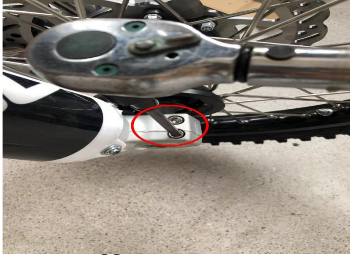
16. Use tool ⑩ to tighten the front shock absorber screw (torque requirement 25-30N.m)
