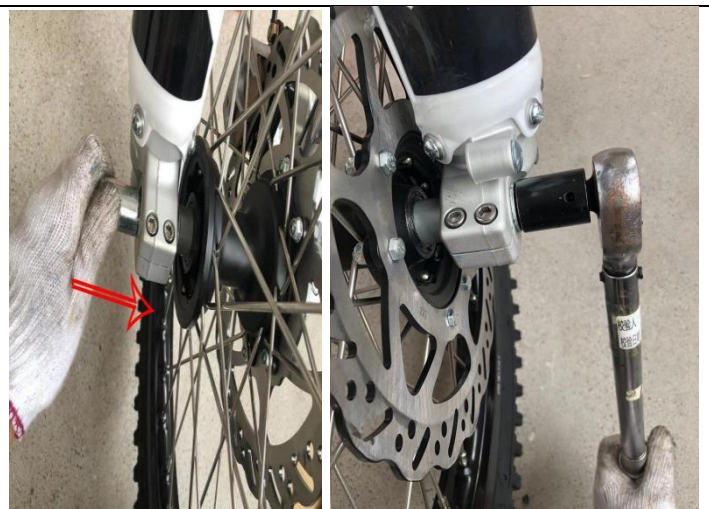
15. Insert the front axle from the right side, then use tool ⑩⑦ to tighten the front wheel fixing nut (torque requirement 80-90N.m) (left long right short for the bush)
