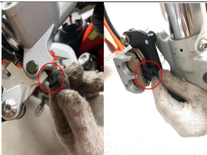
14. Remove the plastic clips of the front disc brake upper & lower cylinder for subsequent installation of the front wheel.
