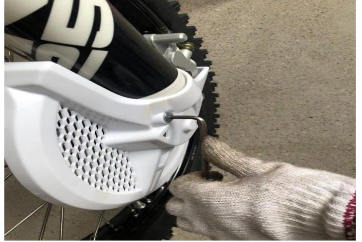
17. Install E to the front left shock absorber and use tool ⑤ to tighten the fixing screws.
