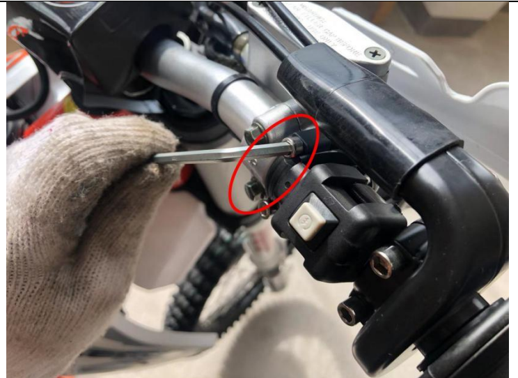
11. Use tool ⑧ to move the front brake upper cylinder to the left of 6-7mm, then assemble D with tool ④ and fix it on the handlebar with tool ⑤
