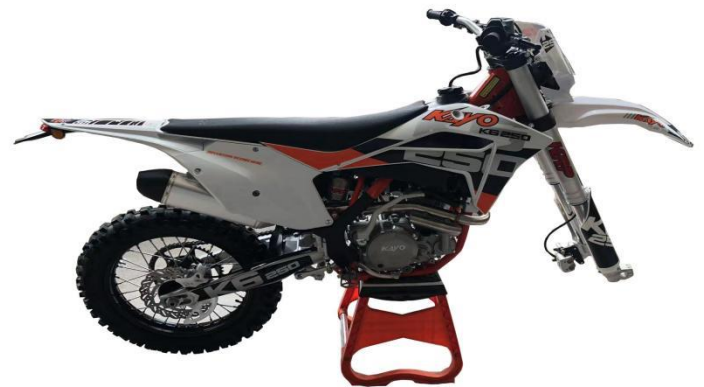
13. Put the vehicle on the stand for easy installation of other accessories.
