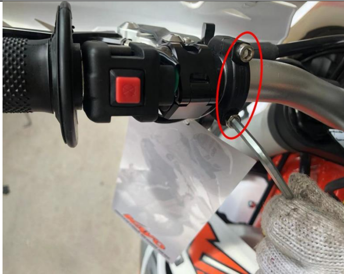
10. Use ④ to assemble D and fix it on the handlebar with tool ⑤
