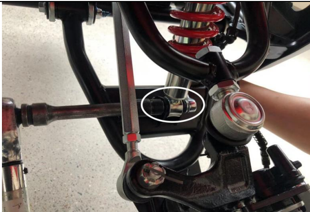
18. Use tool ⑫ to remove the cable fixing the shock absorber, then use ① ② ④ ⑨ to tighten front shock fixing hardware(P) (torque requirement 30-40N.m).
