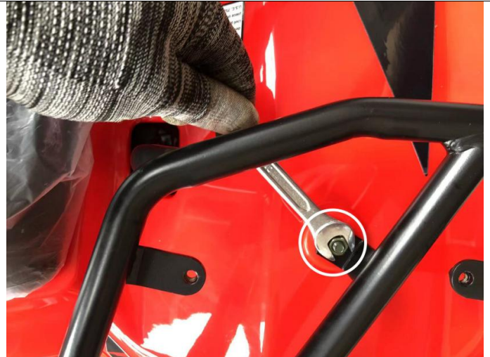
11. Use tools ⑧⑨ to tighten rear rack hardware for rear rack & rear plastics(K).
