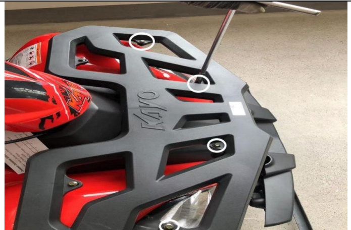
13. Use tool ⑬ to tighten front rack plastic cover hardware (I) (the circles in the picture use M6*16 the rest use M6*12)
