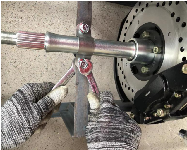
16. Use tools ⑧⑩ to remove the fixing screws of the iron frame.
