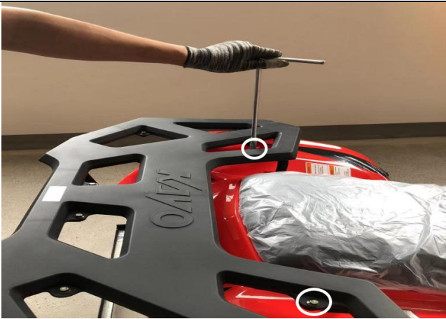
12. Use tool ⑬ to tighten rear rack plastic cover hardware (J) (the circles in the picture use M6*16 the rest use M6*12)
