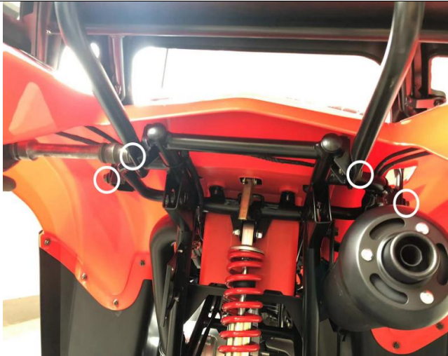
10. Use tools ①②③ to tighten the rear rack screws(M).(torque requirement 25-30N.m)
