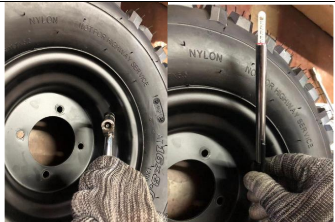
19. Please refer to user's manual (A) for air pressure requirements. Use compressed air to inflate the tires and use the air pressure gauge (B) to inflate to the standard value of 5psi.
